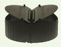
The DraftStoppa® contains a patented mechanism incorporating a pair of balanced flaps which open when the fan is on and close under their own weight when it is off, thus keeping out external air, vermin, dust and odours while reducing energy costs.
